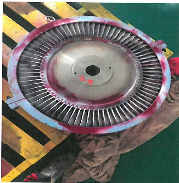
Power Turbine Stage I
