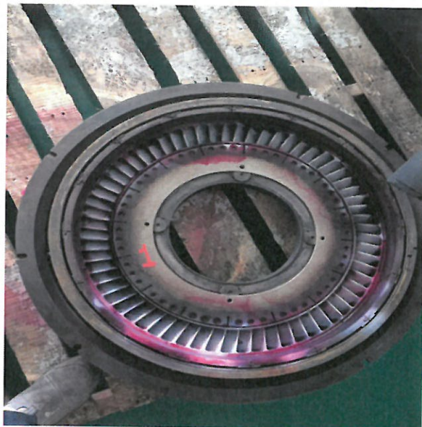
Compressor Turbine Stator Vanes Stage2
